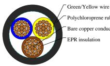
Polychloroprene rubber outer jacket Bare copper conductor EPR insulation
